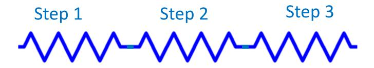
If the resistance of Step 2 is 1 megaohm, and step 1 and step 3 are 1 ohm, the overall resistance is ~ 1 megaohm
